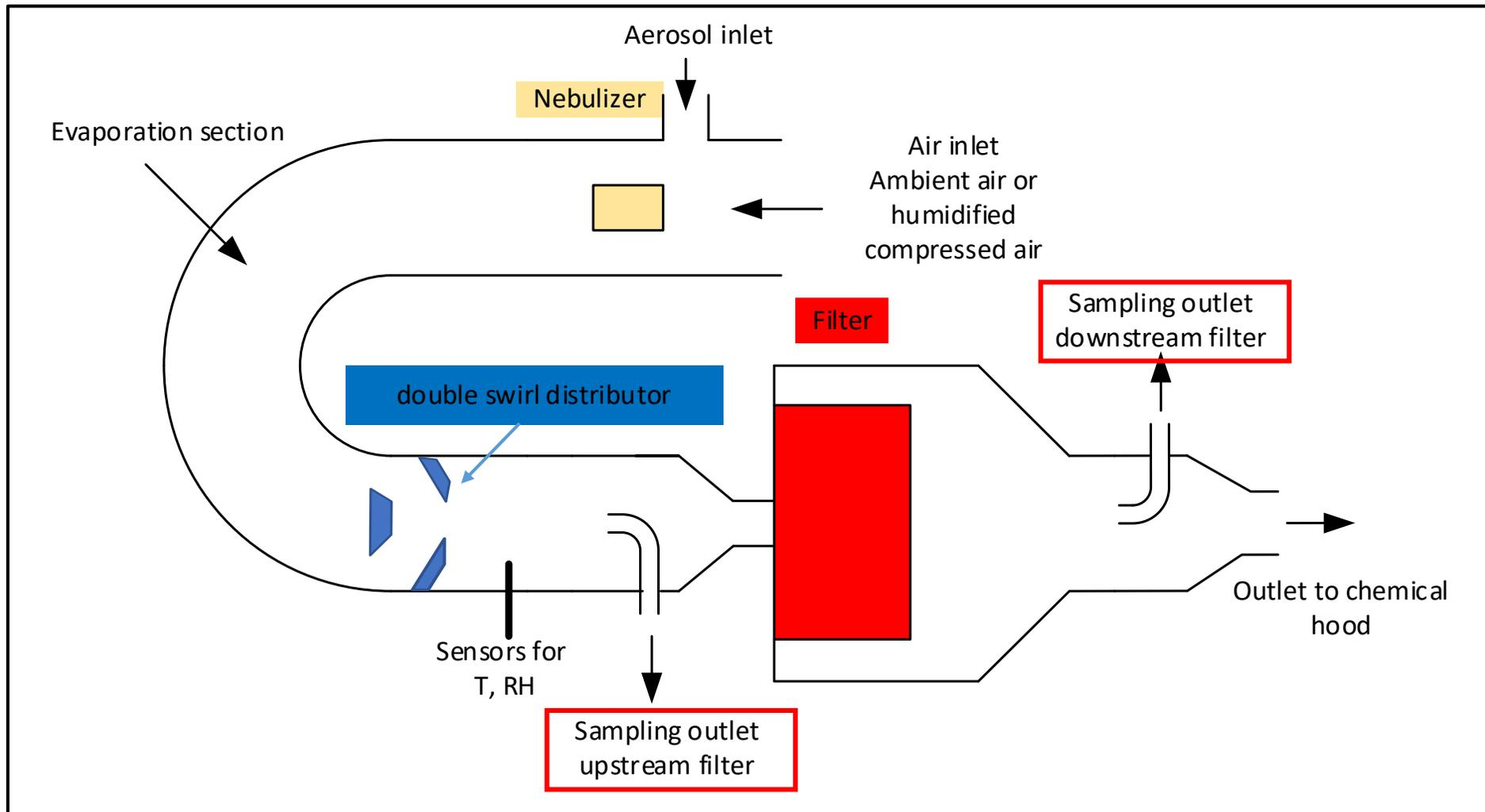
$T = 21^{\circ}\text{C}$ ;  $\text{RH} = 40\text{--}50\%$ ; flow rate  $\approx 20\text{ m}^3\text{ h}^{-1}$  main flow and  $5\text{ L min}^{-1}$  sample flow
