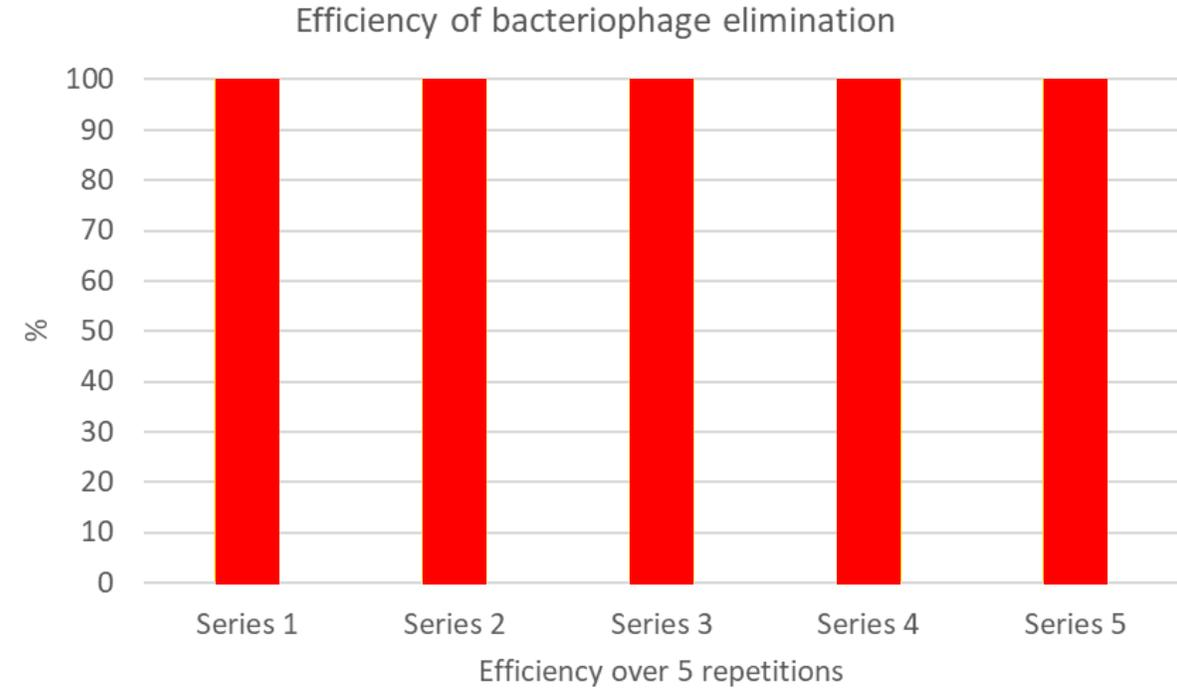
The efficiency of virus (bacteriophage) elimination by NanoCleanAir® filter is > 99% (n=5)
