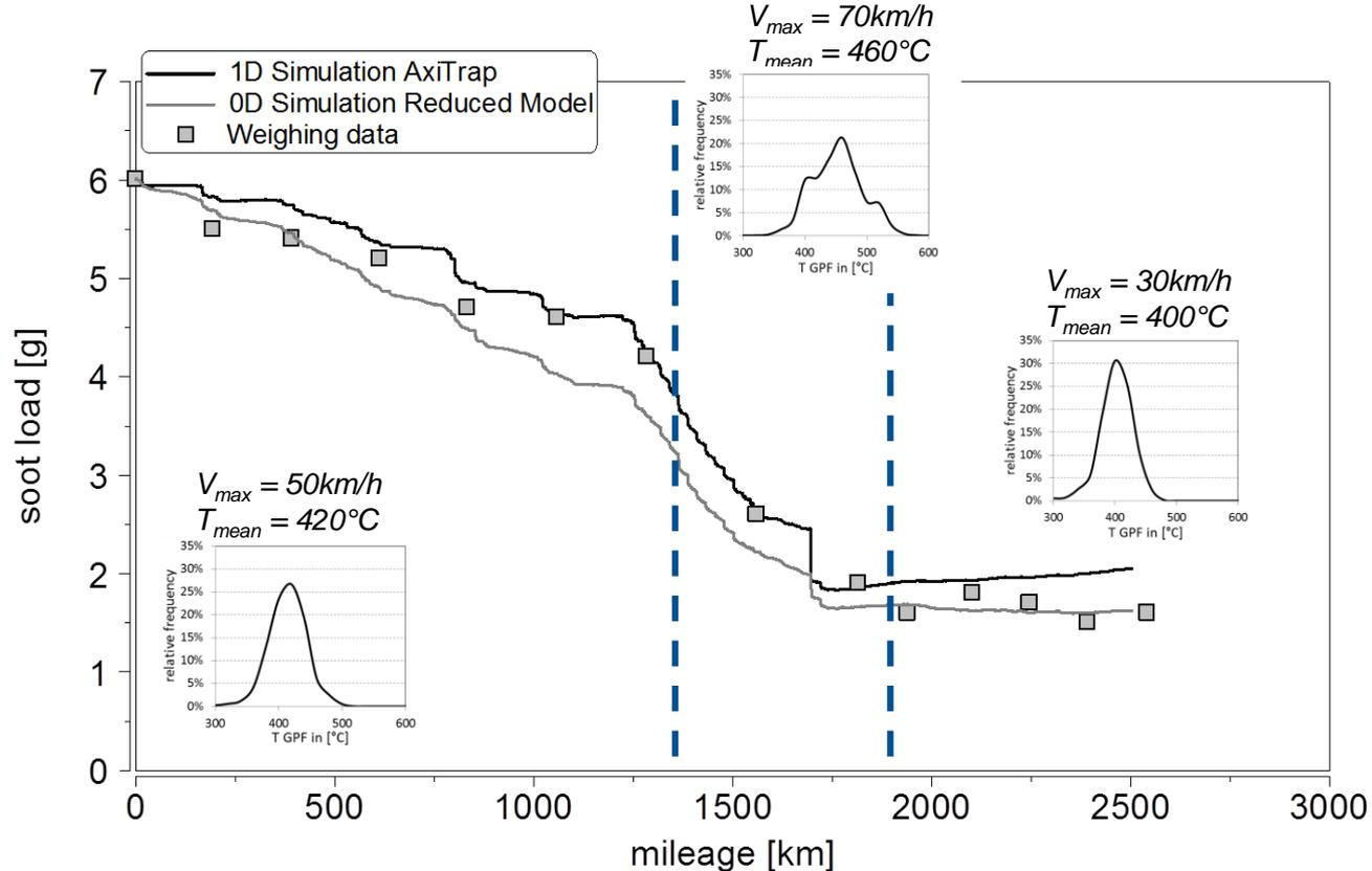
SAE 2015-01-1048, Nicolin et al., "Modeling of the Soot Oxidation in Gasoline Particulate Filters"
