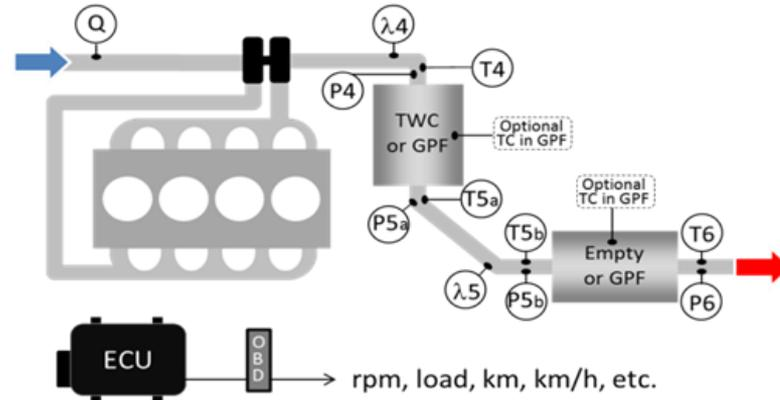
SAE 2015-01-1048, Nicolin et.al., "Modeling of the Soot Oxidation in Gasoline Particulate Filters"
