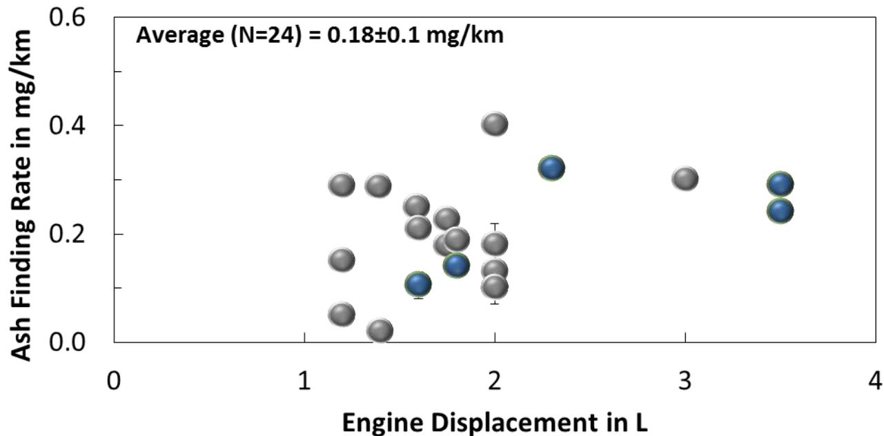
JSAE 2018-5404, Chijiwa et.al., "Ash accumulation in advanced gasoline particulate filter technologies"
