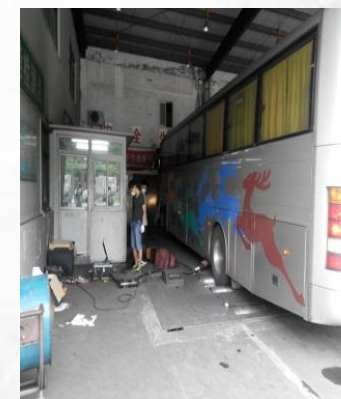
DPF Test on Chassis Dyno.
