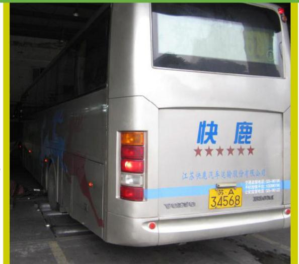
*One of the busses used in the Xia Men project for real driving emission and chassis dynamometer measurements*
