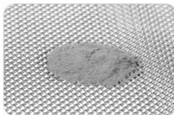
Step 2: The pourable powder mix is applied to reinforcing expanded metal
