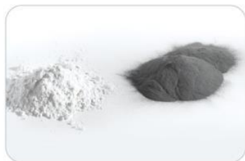
Step 1: For further processing the high alloy metal powder is mixed with a binder
