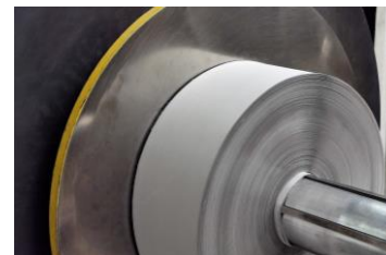
Step 4: SMF® medium is sintered in two steps and is available for further processing on coils with 170 m material length
